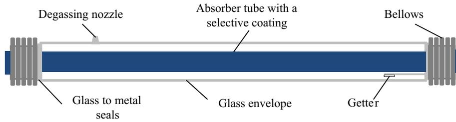
Fig. 1. Schematic of a typical parabolic trough receiver.
