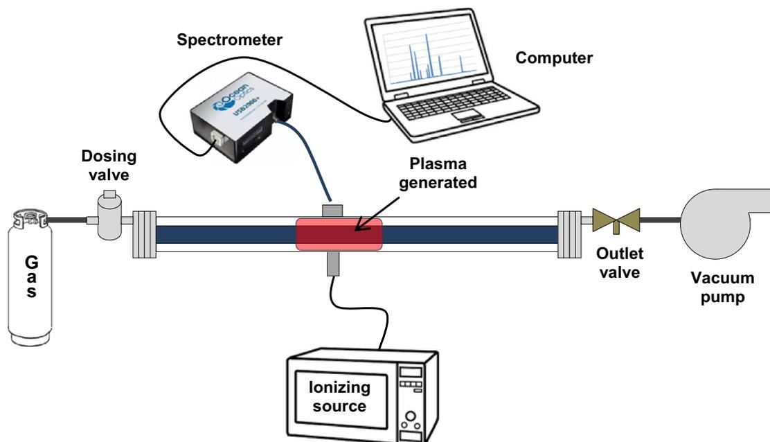
Fig. 2. Experimental set-up for AGA calibration.
