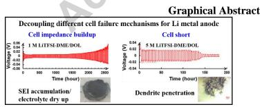
The conflicting requirements on SEI properties towards preventing the continuous Li dendrite growth and mitigating impedance accumulation are discussed and quantified for Li metal anode. A broadly applicable fundamental rule has been discovered to understand the morphology evolution of Li metal in different electrolytes, providing fundamentally new insights for addressing challenges in rechargeable Li metal batteries.
