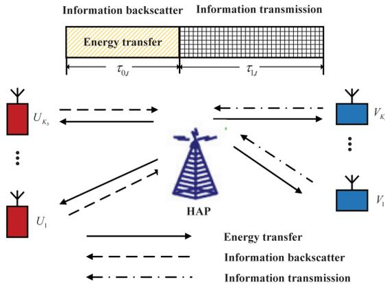
**Fig. 1** Backscatter assisted wireless powered communication network with NOMA.
