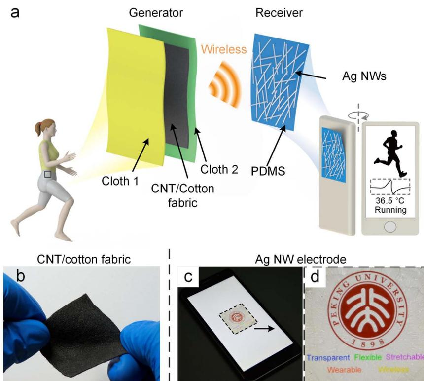
**Fig. 1.** Structure of self-powered wireless smart patch. (a) Schematic diagram of a self-powered wireless smart patch. (b) Photograph of the stretchable conductive fabric after coating PDMS. (c), (d) Transparent and stretchable Ag NW/PDMS electrode pasted on the screen of a smart phone.
