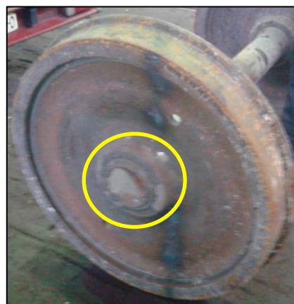
Fig. 2. The railway wheel and axle with signed fractured surface
