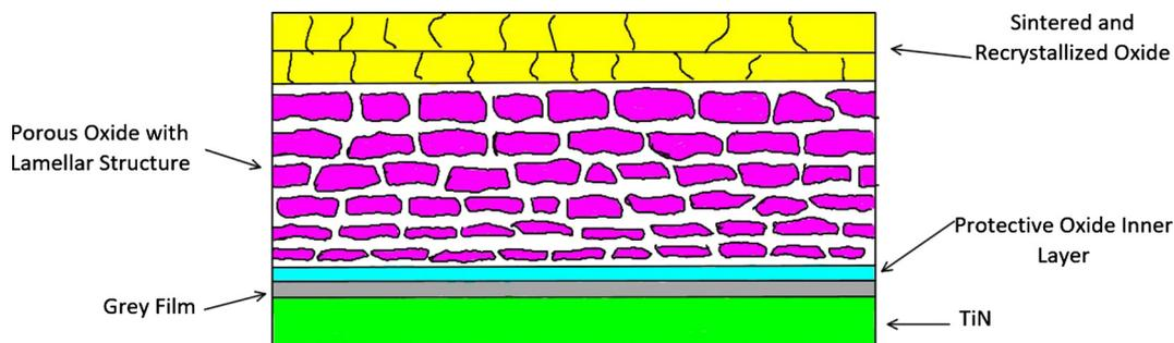
Fig. 1. Schematic of the cross section of the oxide scale structure on  $\text{TiN}$  [8].
