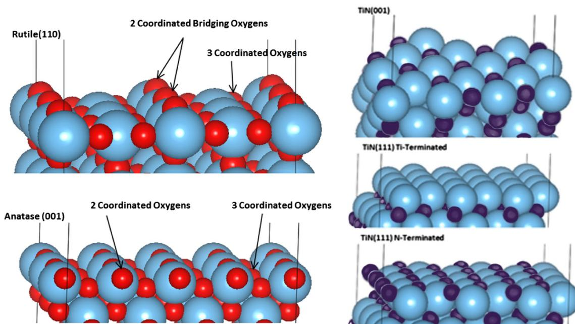
Fig. 2. Relaxed  $\text{TiO}_2$  and  $\text{TiN}$  surfaces used to construct  $\text{TiN}/\text{TiO}_2$  interfaces; Titanium (Blue), Oxygen (Red), Nitrogen (Purple). (For interpretation of the references to colour in this figure legend, the reader is referred to the web version of this article.)
