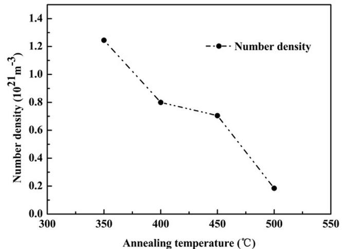
Fig. 2. Number density of dislocation loops as a function of annealing temperature in hydrogen ion implanted iron.
