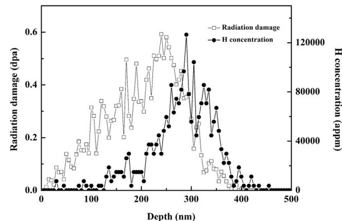
Fig. 1. SRIM calculation of irradiation damage and H concentration profile in hydrogen ion implanted pure iron.
