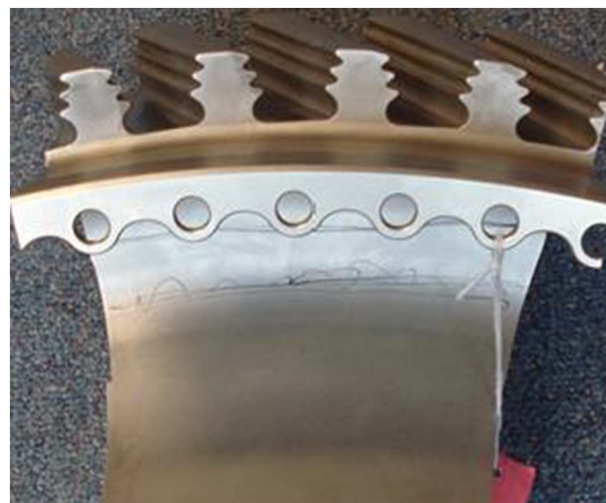
Fig. 1. An as-received section of the Inconel-718 disc with broached and shot-peened fir-trees.
