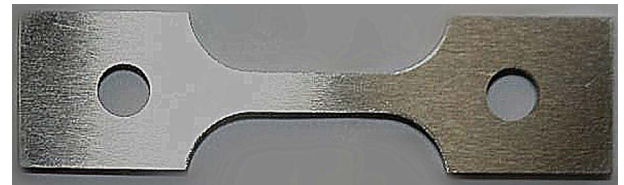
Fig. 3. Creep specimen without film-holes.
