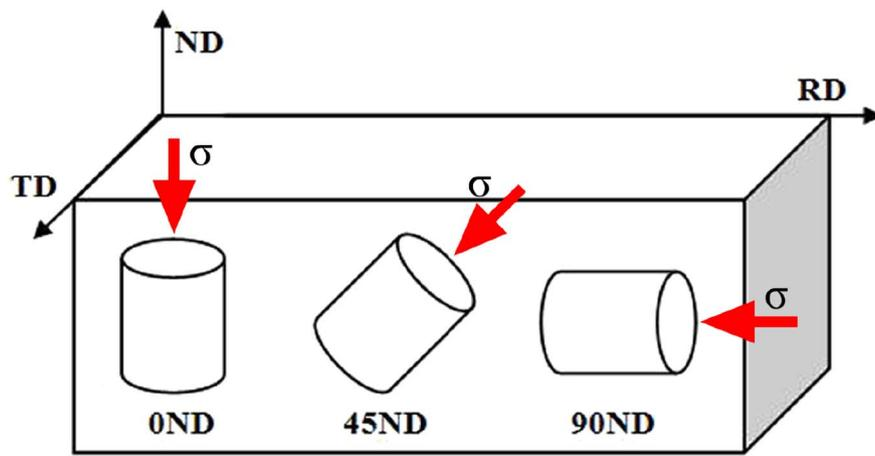
Fig. 2. Schematic illustration of the samples used for compression tests.
