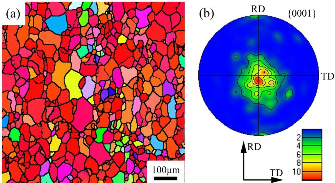
Fig. 1. The as-received AZ31 Mg alloy sheet: (a) Orientation map and (b) {0001} pole figure.
