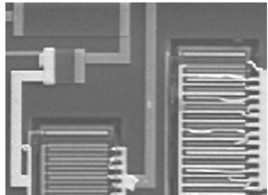
Fig. 4. SEM images of a B type device: details show a very bad adhesion between gold and tungsten layers.
