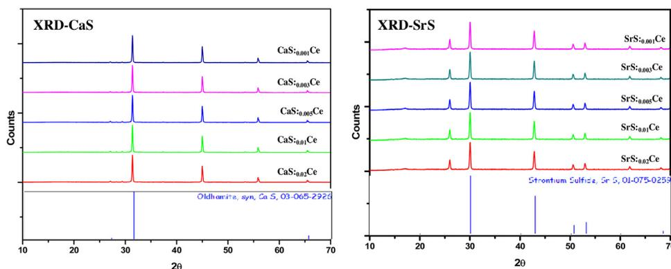
**Fig. 1.** XRD patterns of CaS and SrS phosphor doped with different concentration of  $\text{Ce}^{3+}$  ions matching with ICDD files (shown as bottom spectra). The lack of response with  $\text{Ce}^{3+}$  addition demonstrates the substitution of Ca and Sr sites.
