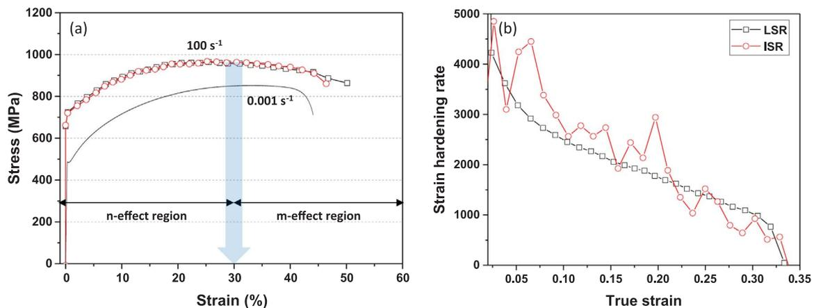
Fig. 2. (a) Tensile stress-strain curve at low and intermediate strain rate, and (b) strain hardening rate curve. CoCrFeMnNi HEA shows higher strength and extended post-elongation at intermediate strain rate without increase in hardening rate.
