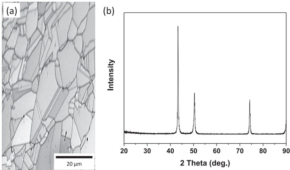
Fig. 1. (a) EBSD image quality (IQ) map and (b) XRD of initial microstructure.
