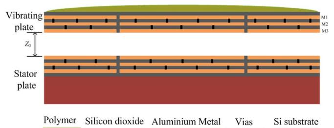
Fig. 2. Cross section view (A–A) of the CMOS–MEMS device with polymer coating on top of the vibrating plate.
