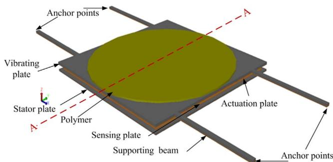
Fig. 1. Schematic of the proposed device.
