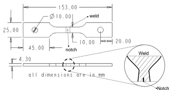
Fig. 1. Geometry of surface flaw type specimen used for fatigue testing.
