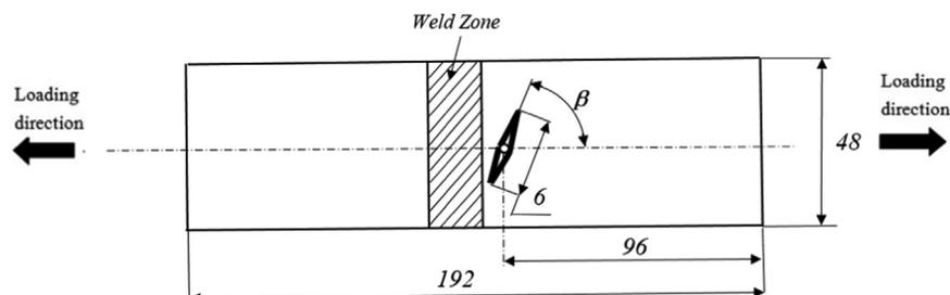
Fig. 1. Center-cracked fatigue specimen (mm).
