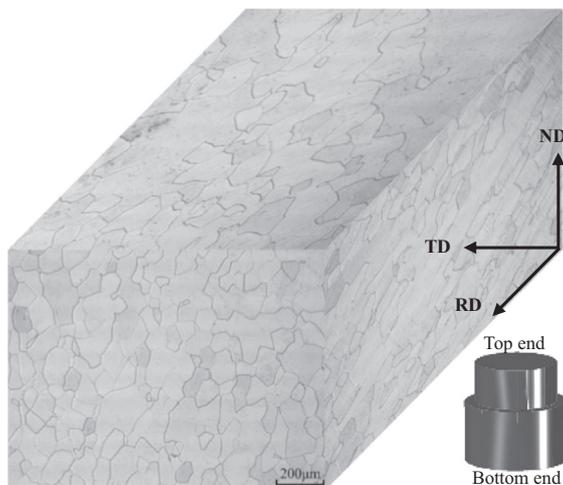
Fig. 1. Microstructure of the initial hot-rolled Ti-5Mo-5V-8Cr-3Al alloy plate. ND, RD and TD respectively stand for the normal direction, rolling direction and transverse direction of the hot-rolled plate.
