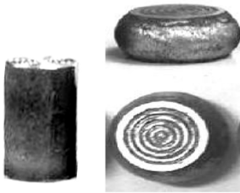
Fig. 1. left side: cylindrical sample before the hot compression test, right side: deformed sample after hot compression.
