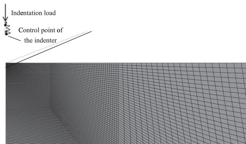
Fig. 2. Finite element model of the sharp indentation with the system compliance included.
