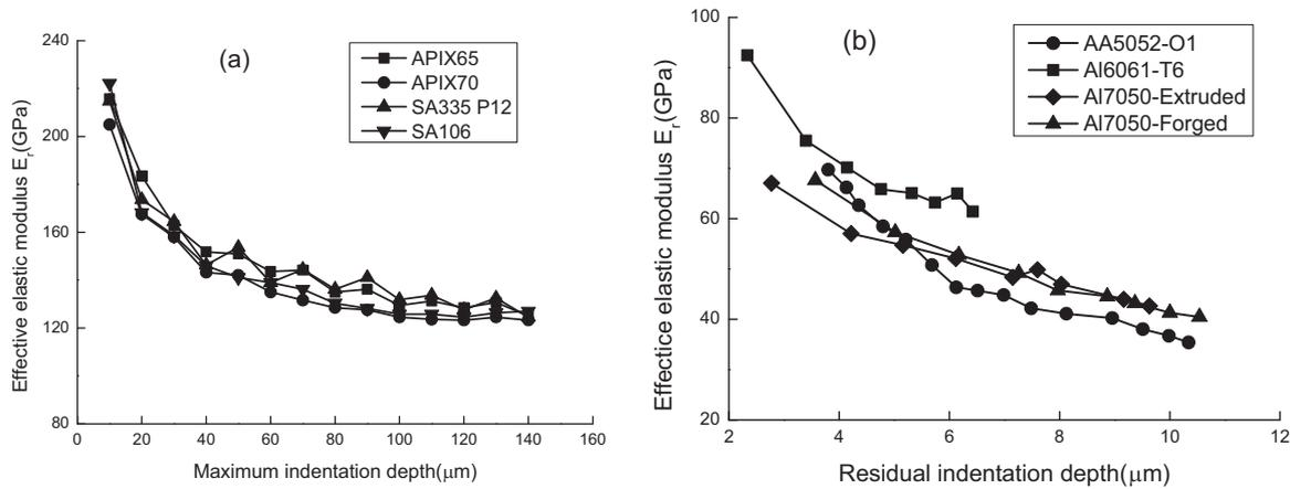
Fig. 1. Measured elastic moduli of steels (a) and aluminum alloys (b) decrease with the indentation depth.
