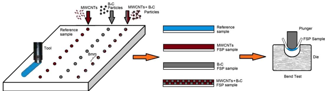
**Fig. 1.** Schematics of the friction stir processing representing the surfaces composites and bending test.
