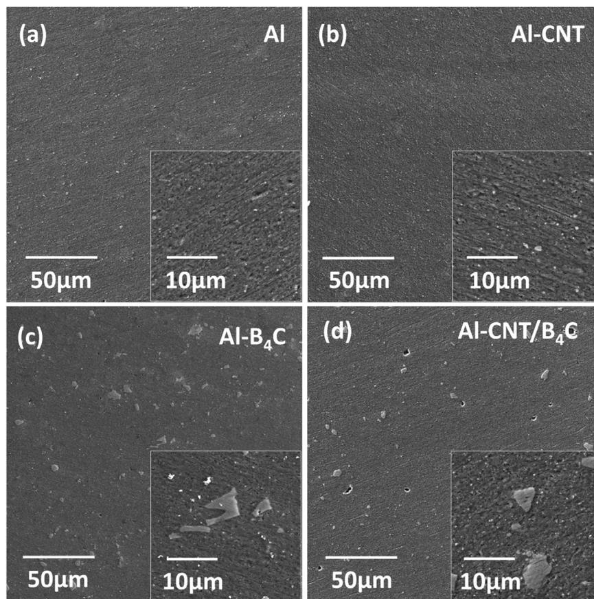
**Fig. 2.** SEM images of FSP reference sample and surface composites: (a) Al5083, (b) MWCNTs in Al5083, (c)  $B_4C$  particles in Al5083 and (d) Hybrid combination of MWCNTs and  $B_4C$  particles in Al5083.
