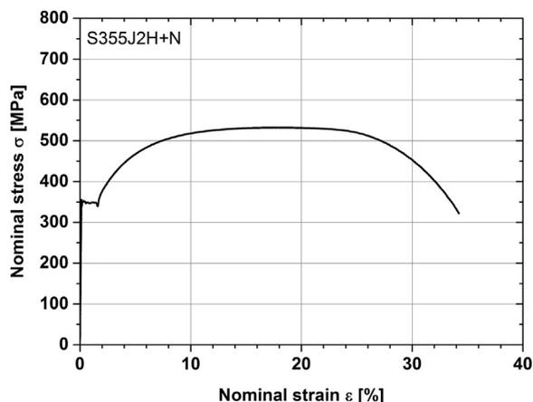
Fig. 1. Nominal stress-strain curve of the base material.
