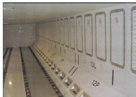
Fig. 1. a-Gillfab 4422 panel, b-cargo compartment lining in sidewalls, ceilings, partition walls and as decompression panels in the lower cargo hold in Airbus A319/A320/A321.
