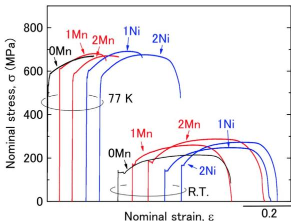
Fig. 1. Nominal stress–strain curves from 1Ni, 2Ni, 0Mn, 1Mn, and 2Mn tested at 77 K and RT.
