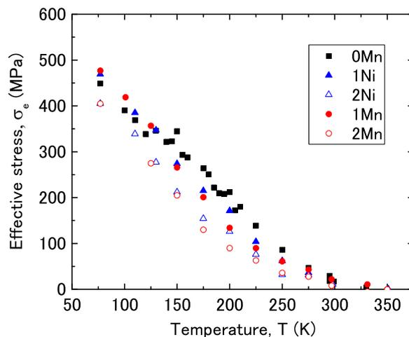
Fig. 3. Temperature dependence of the effective stress.
