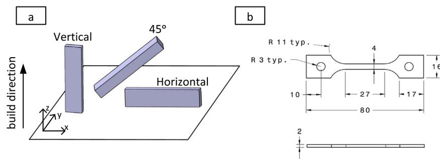
Fig. 1. (a) Specimen orientations during processing; (b) Tensile specimens (dimensions in mm).
