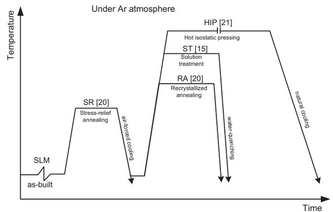
Fig. 2. Specimens designation and corresponding thermomechanical treatment (TMT) routes.
