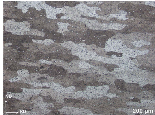
Fig. 1. Optical photomicrograph of the initial microstructure of AA 2219-T87 plate used in the present study. The plate rolling and normal directions are shown. The microstructure consists of grains with clear grain boundaries that are slightly elongated in the direction of rolling. Bright particles seen in the microstructure are primary CuAl 2 particles uniformly distributed throughout.
