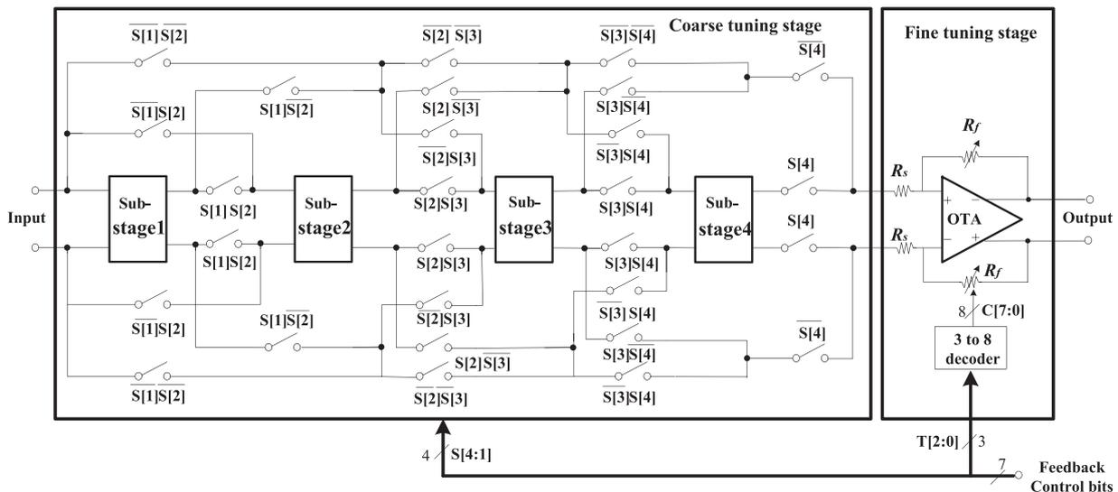
Fig. 3. VGA structure employed in this work.
