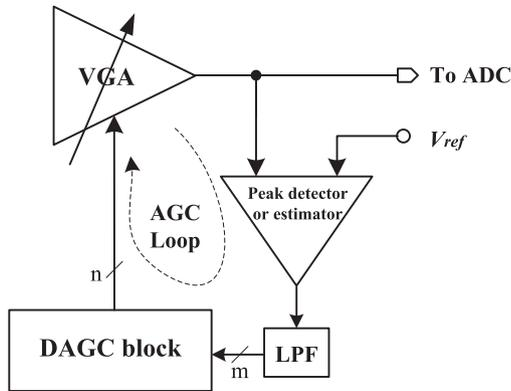
Fig. 1. Architecture of a typical feedback AGC loop.
