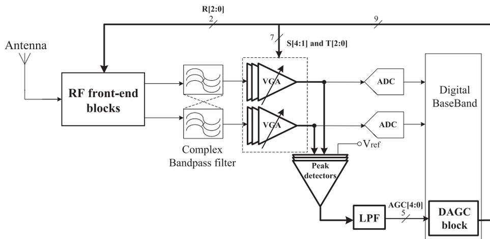
Fig. 2. Block diagram of proposed AGC loop inside the ZigBee receiver.
