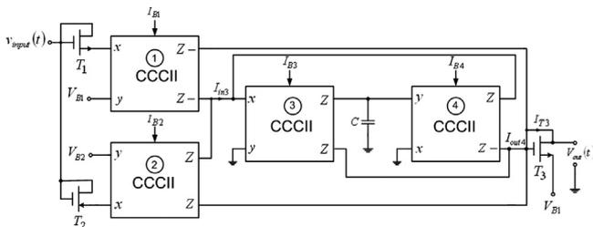
Fig. 1. The proposed circuit of the peak detector.
