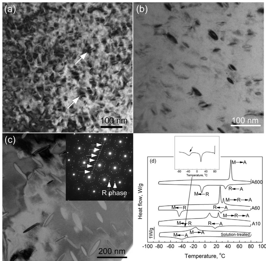
**Fig. 1.** TEM bright field images of the aged samples, (a) A10, (b) A60 and (c) A600. Diffraction patterns corresponding to the  $[111]_{\text{B2}}$  were also inserted, respectively. DSC curves of the solution-treated and aged samples are shown in (d). The transformation sequences are also indicated.
