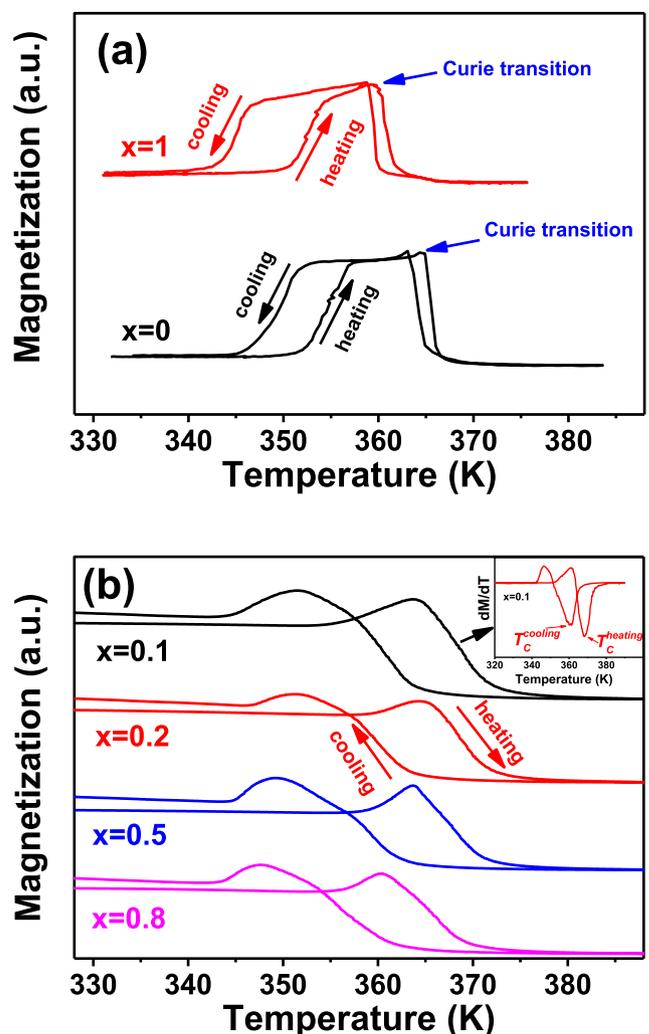
Fig. 1.  $M-T$  curves of  $\text{Ni}_{50-x}\text{Tb}_x\text{Mn}_{30}\text{Ga}_{20}$  ( $x = 0-1$ ) alloys measured under a magnetic field of 500 Oe. (a)  $x = 0$  and 1; (b)  $x = 0.1-0.8$ . The inset in (b) is the differential curve for  $x = 0.1$  alloy.
