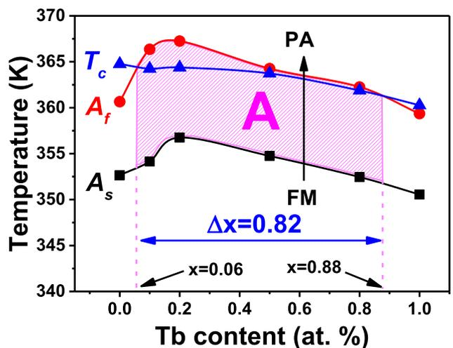
Fig. 2. Vertical phase diagram of  $\text{Ni}_{50-x}\text{Tb}_x\text{Mn}_{30}\text{Ga}_{20}$  ( $x = 0-1$ ) alloys. FM and PA in the figure represent ferromagnetic martensite and paramagnetic austenite, respectively.
