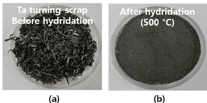
Fig. 1. Images of Ta turning scrap (a) before and (b) after hydridation at 500 °C and milling processes.
