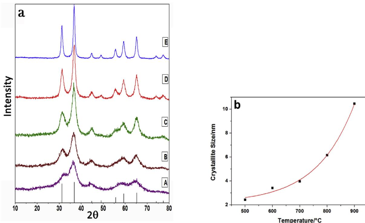
Fig. 1. (a) XRD patterns of Cr-doped ZnAl<sub>2</sub>O<sub>4</sub> rapid-annealed at different temperatures and (b) plot showing the variation in crystallite size with temperature.
