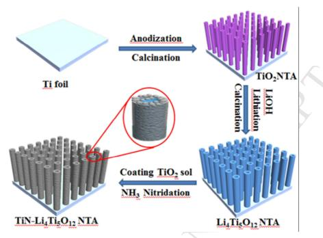
A schematic showing the preparation process of  $TiN-Li_4Ti_5O_{12}$  NTA via anodization oxidation, lithiation, surface coating  $TiO_2$  and nitridation treatment.
