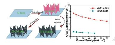
Interconnected Ni-Co sulfide nanosheet arrays directly grown on nickel foam exhibits ultrahigh areal capacitance for supercapacitors.
