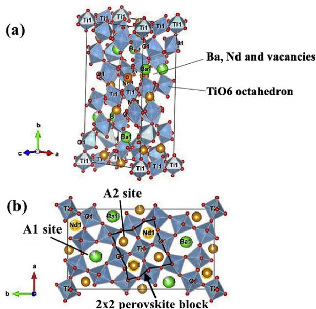
Fig. 1. Schematic representation of (a) Ba<sub>3.75</sub>Nd<sub>9.5</sub>Ti<sub>18</sub>O<sub>54</sub> with tungsten-bronze type like structure and (b) the c-axis was chosen as the short axis.
