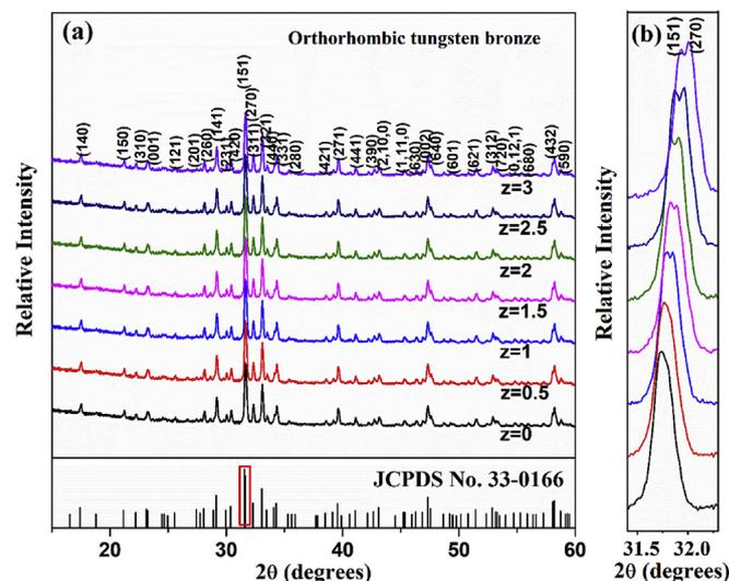
Fig. 2. (a) XRD patterns of BNT-(AN)<sub>z</sub> ( $z = 0-3$ ) ceramics sintered at 1375 °C for 4 h in air. (b) The characteristic peaks of (270) and (151) for BNT-(AN)<sub>z</sub> phase of corresponding samples.
