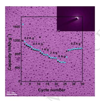
Amorphous  $Fe_2O_3$  nanospheres anchored on reduced graphene oxide ( $Fe_2O_3/rGO$ ) were prepared by the electron beam radiation approach. The  $Fe_2O_3/rGO$  exhibits a highly reversible capacity of 1064 mA h g<sup>-1</sup> after 100 cycles at 200 mA g<sup>-1</sup> with 88% of capacity retention and a superior rate capacity of 580 mA h g<sup>-1</sup> at 5000 mA g<sup>-1</sup> for Li ion storage.
