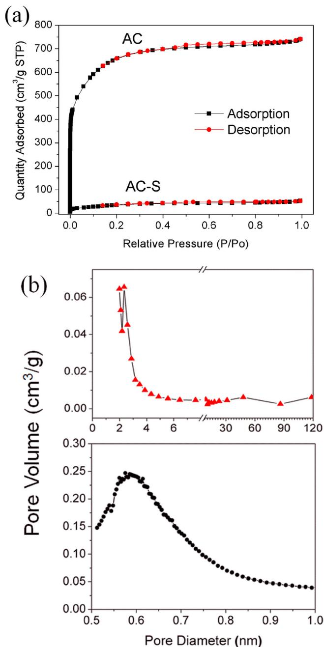
Fig. 2. (a)  $N_2$  adsorption-desorption isotherms and (b) BJH pore distribution of AC.
