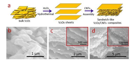
Sandwich-like structure hefero-structured Vanadium Pentoxide/carbon nanotubes complex is prepared via hydrothermal method and self-assembly process.
