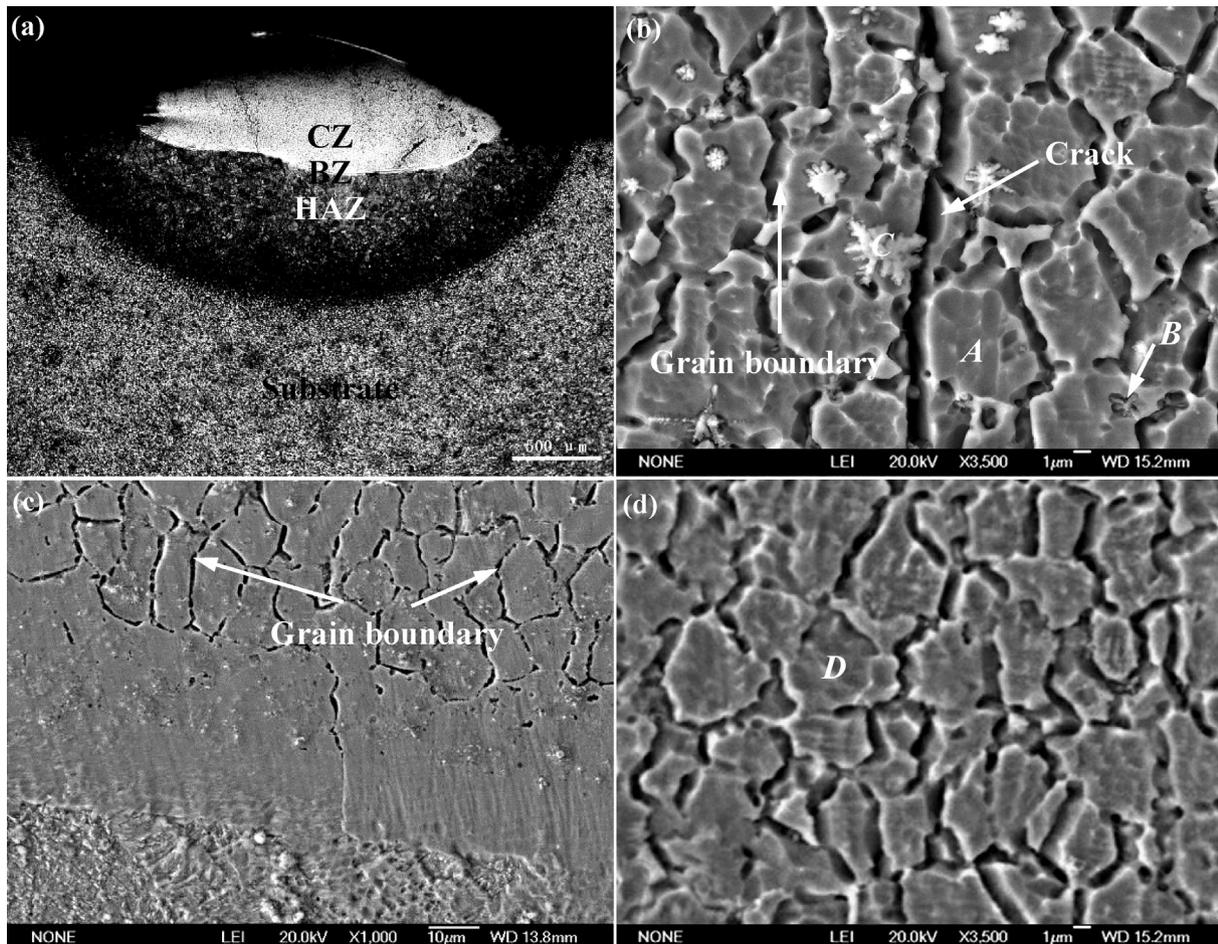
Fig. 1. Micrographs of the high-entropy alloy (a) macroscopic feature of  $\text{Co}_{0.5}$  alloy, (b) cladding zone of  $\text{Co}_{1.5}$  alloy, (c) bounding zone of  $\text{Co}_{0.5}$  alloy, (d) cladding zone of  $\text{Co}_{2.0}$  alloy.
