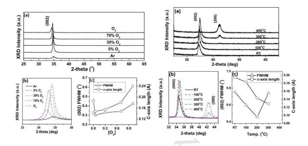
XRD characterization results of the ZnMgO films grown under different oxygen partial pressures; (a) XRD full scan spectra, (b) high resolution (0002) XRD peaks, (c) c-axis parameters and the FWHMs of the (0002) peaks
