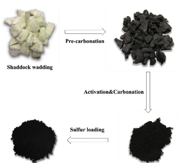
**Scheme 1.** Schematic plot for the fabrication of SWD–S composite.
