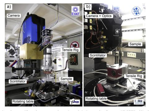
Fig. 2. Experimental setup used for synchrotron tomography experiments during interrupted tensile tests at a) ID15/ESRF and b) at P05/PETRAIII.
