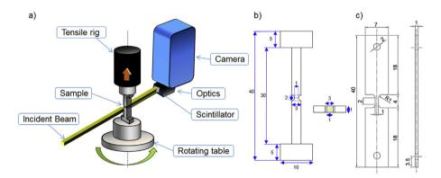
Fig. 1. a) schematic representation of the setup used for the interrupted tensile tests and geometry of the samples used at b) the ID19 and ID15 beamlines of the ESRF and c) P05 of PETRA III.
