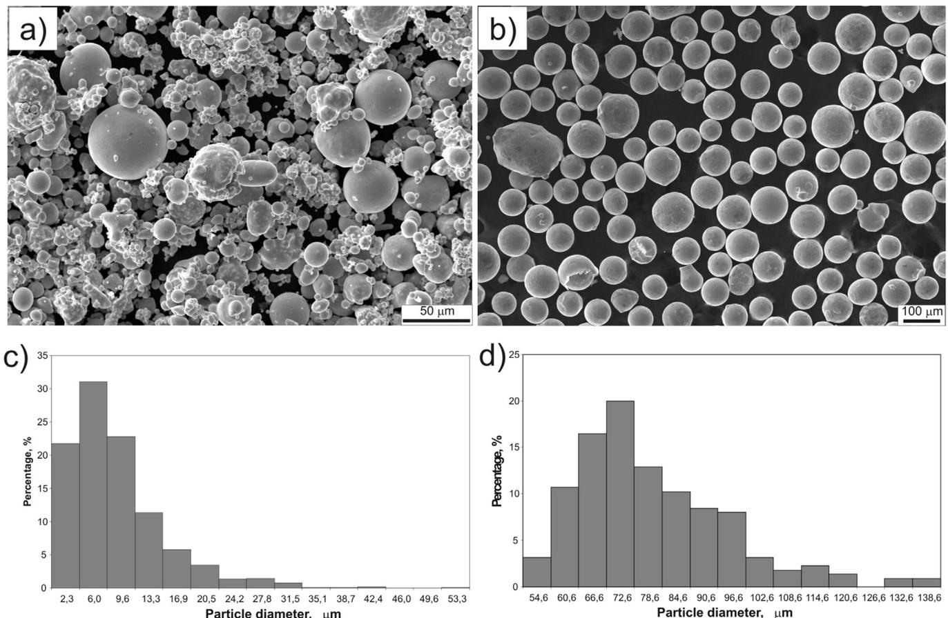
**Fig. 1.** Powders in as-received state: a) water atomized Ag powder, b) 1559-40 powder, c) particle size distribution of the Ag powder, d) particle size distribution of the 1559-40 powder.
