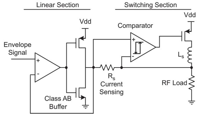
Fig. 2. Push amplifier block diagram [12].
