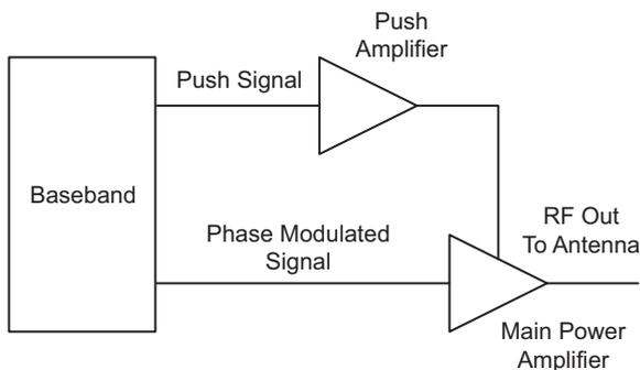
Fig. 1. Envelope tracking power amplifier block diagram.
