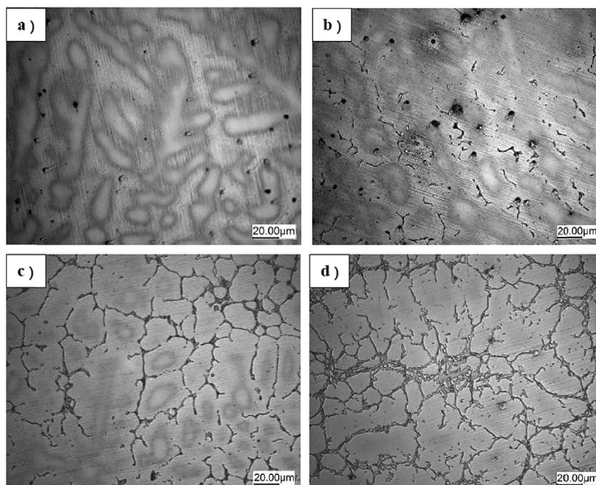
Fig. 1. Optical micrographs of solution treated  $\text{Ni}_{50}\text{Mn}_{36}\text{Sn}_{14}$  alloys with adding different amount of Gd, and the amount of Gd addition is (a) 0; (b) 0.5 at.%; (c) 1 at.%; (d) 2 at.%.
