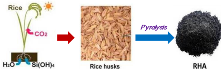
Scheme 1. Preparation of Rice husk ash
