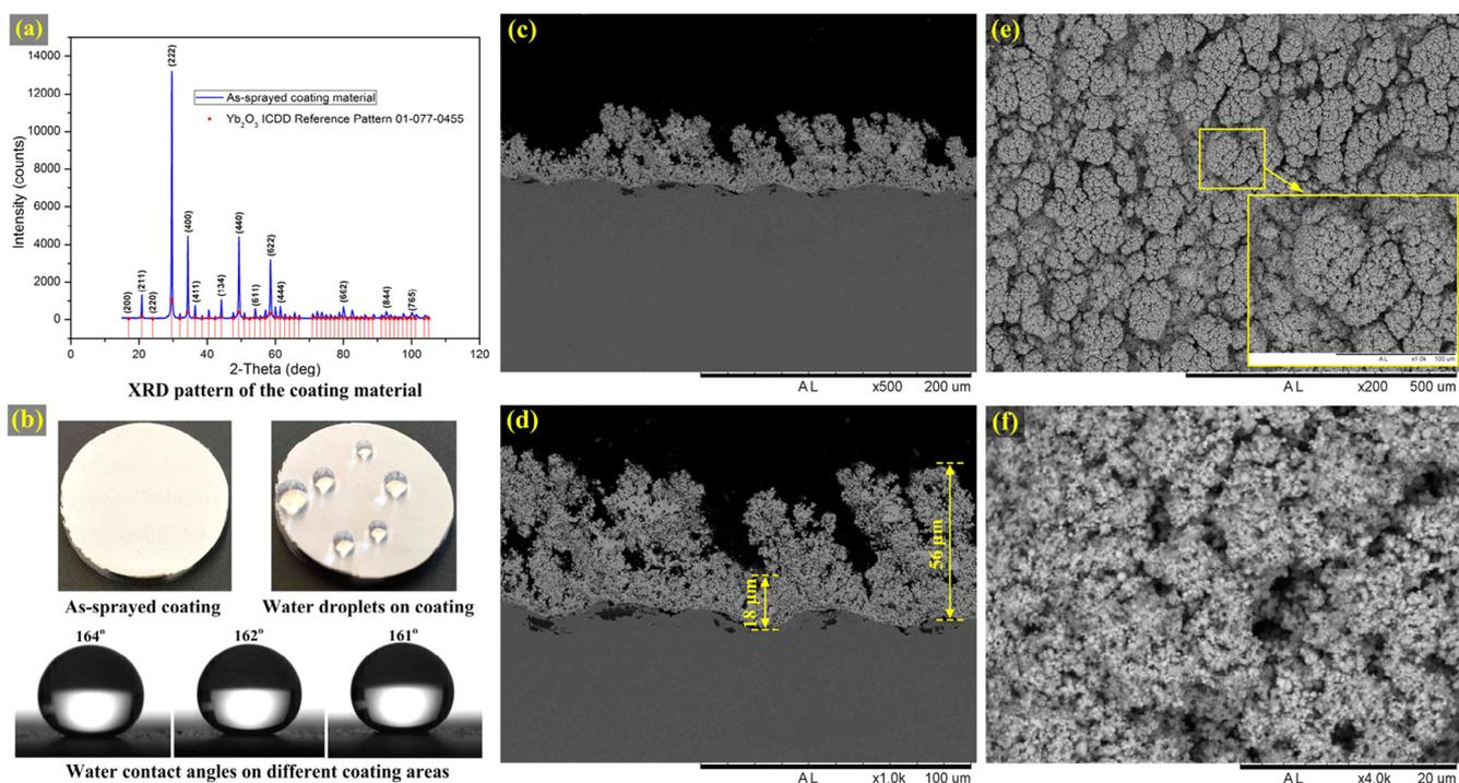
**Fig. 1.** (a) XRD pattern of the coating material; (b) Water droplets on the coating and WCA measurement; (c, d) Cross sectional microstructure; (e, f) Top surface microstructure.
