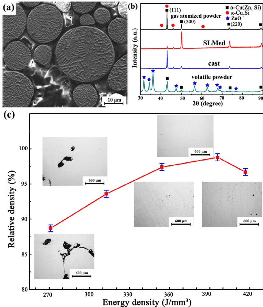
**Fig. 1.** (a) Cross-section morphology of the atomized powder. (b) XRD patterns of atomized powder, SLM-produced and cast specimens, and volatile substance. (c) Relative density and corresponding optical images of the SLM-produced samples.
