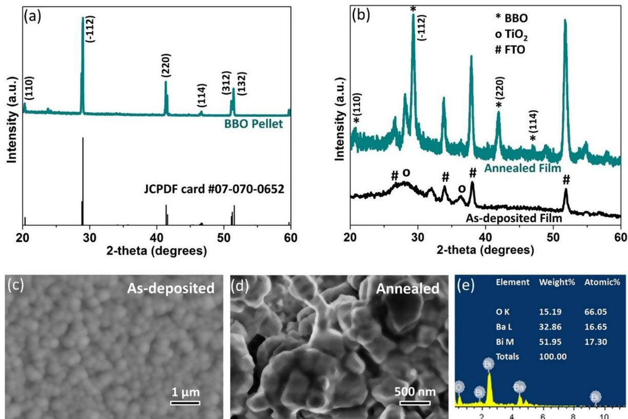
**Fig. 1.** (a) XRD pattern of phase pure BBO pellet. (b) XRD pattern of BBO thin-film deposited by PLD on TiO<sub>2</sub>/FTO Stack, before and after annealing (c) SEM image of as-deposited thin-film (d) SEM image of annealed BBO thin-film (e) EDS spectra for annealed BBO thin-film, showing the expected stoichiometry.
