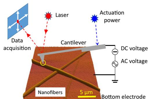
Fig. 1. Experimental setup for the measurement of the piezoelectric response of single nanofibers (the nanofibers in the figure is real).
