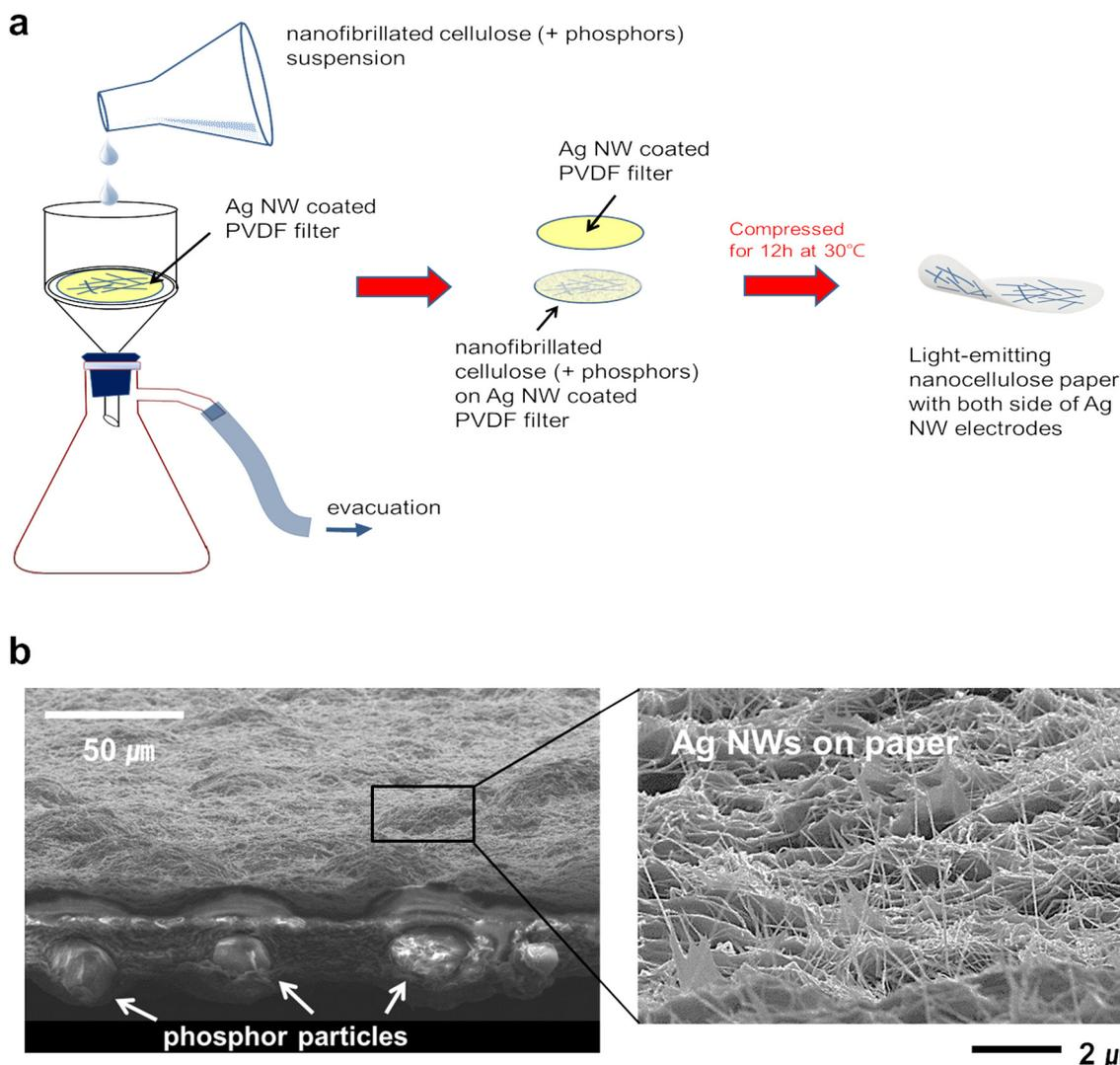
**Fig. 1.** (a) Schematic illustrations of the fabrication of a light-emitting transparent NCP. (b) Scanning electron microscopic images of the cross-section and the surface high-resolution of light-emitting transparent NCP.
